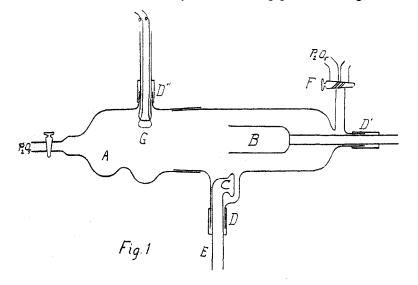
to obtain an atmosphere dry enough to make the transfer without hydrolysis. In order to detect possible hydrolysis after the transfer had been made, the two-way stopcock F was turned and the air within the apparatus was run into a solution of silver nitrate.
